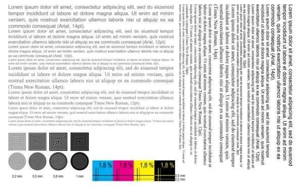
Figure 2: Test form, with test patterns and Ecofont software-processed Arial and Times New Roman on the left side, and text with respective conventional fonts on the right side
