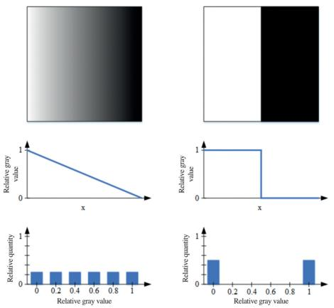
Figure 1: Blurred and sharp edges (left and right, respectively) and their corresponding brightness distribution
