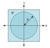
Figure 4: Frame Ψ (hatched area) with low limit frequency b, which is used in the FFT in order to concentrate on high frequencies
