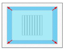
Figure 12: Sensor filling stroke pattern (left) and windowed stroke pattern (right); the acquisition area in the lowermost camera position is highlighted in light blue, in the uppermost position in blue, the red arrows mark the enlargement of the acquisition area
