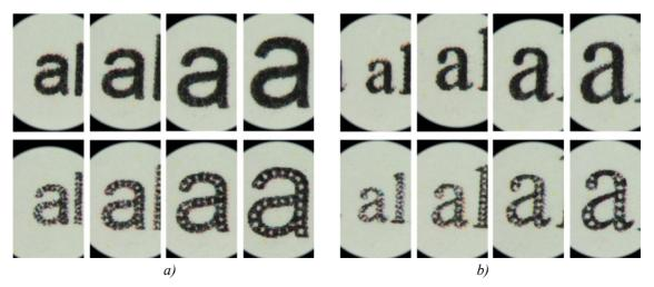
Figure 5: Photographs of letter 'a' in all four sizes printed with EF: (a) Arial, (b) Times New Roman; first row: unprocessed text, second row: Ecofont software-processed text
