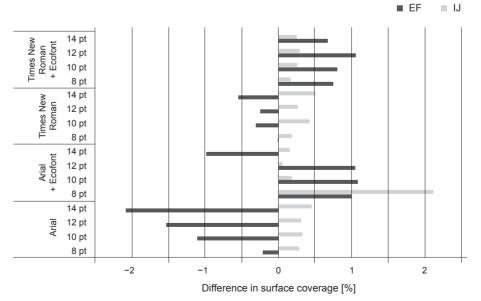
Figure 8: Differences in surface coverage of digital form of letter 'a' and printed letter 'a' between prints made with the printers IJ and EF before and after ageing
