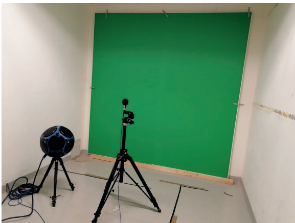
Figure 2: One of the printed plates mounted on the wall in the reverberation room; the omnidirectional loudspeaker and microphone are also shown
