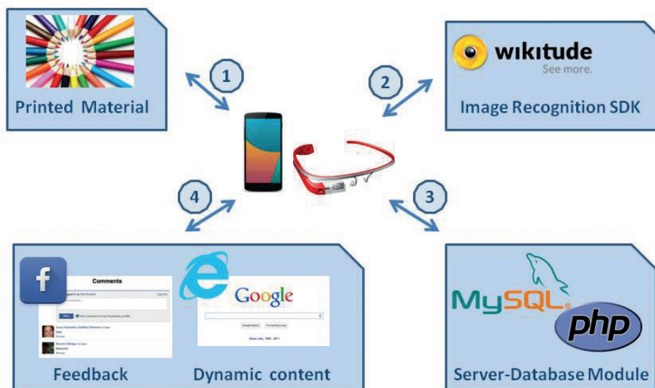
Figure 2: User interaction and image recognition with the RocReadaR app.: 1) The user runs our application on an Android smart device and points it at a printed document with the relevant media already linked with it, this media is stored on our server and is defined on our database; 2) The Wikitude SDK then helps to recognize if the print content is pre-defined or not, by using .WTC 'tracker' file that was generated when we stored the data, and by comparing the image signatures in the tracker, the SDK returns a match/miss result; 3) If a match occurs, we search for the mapping of print document to relevant media on the Server-Database Module and return this information to the Android device; 4) Using the response from the server database module and metadata of relevant media we present Web and Social media in an augmented environment on the Android device
