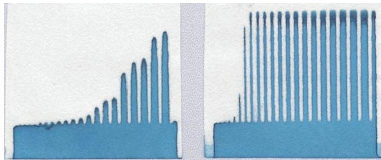
Figure 8. Examples of channel tests, printed on Whatman 4 filter paper with AKD ink at a drop spacing of 45 μm (left) and with PS ink at a drop spacing of 15 μm (right)
