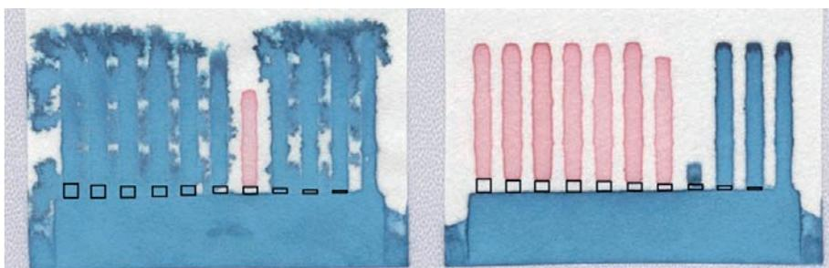
Figure 6: Reverse side views of the samples shown in Figure 5; on Whatman 1 (left), significant liquid spreading on the reverse side can be observed; barriers have been outlined with rectangles, as in Figure 5
