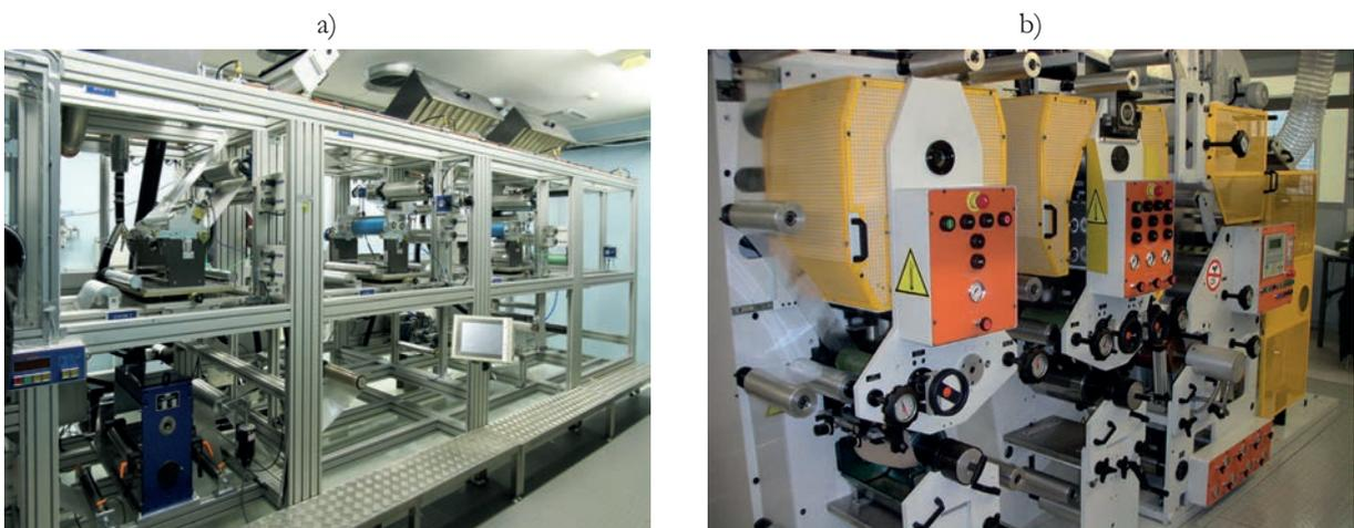
Figure 1: a) Pilot machine used for rotary screen printing of conductive micro-particle pastes and insulator materials;
