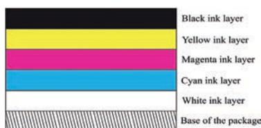
Figure 1: Geometry of a package structure printed with the CMYK model along with a white background (WCMYK)
