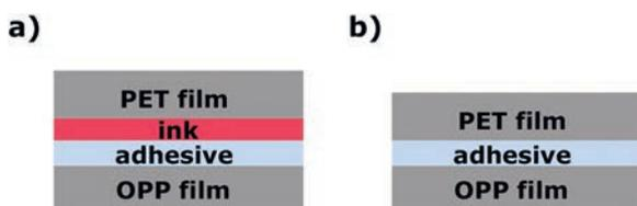
Figure 1: The structure of the laminates used for the tests, a) printed, b) unprinted
