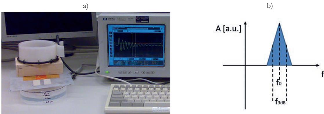
Figure 4: a) Measurement setup for the analysis of the resonance frequencies and  $Q$ -values of the printed sensors at moist and dry conditions; the sensor is separated from the water source by 4 cm thick dry Finnish pine wood; b) Definition of  $Q$ -factor in frequency domain
