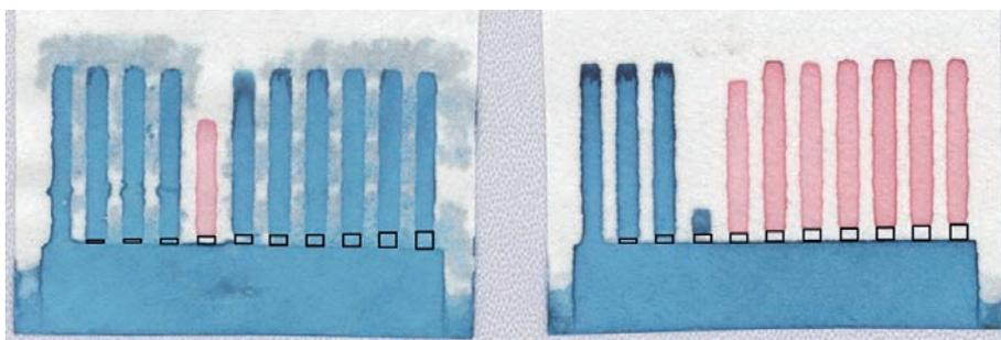
Figure 5: Examples of barrier tests, printed with PS ink at drop spacing of 15  $\mu\text{m}$  on Whatman 1 (left) and Whatman 4 (right) filter papers; for clarity, printed barriers have been outlined with rectangles
