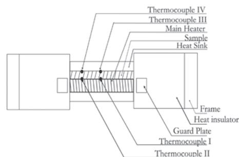
Figure 2: Schematic diagram for the measurement of thermal conductivity of different ink samples
