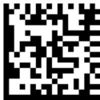
Figure 2: Data Matrix encoding a web link to Google
