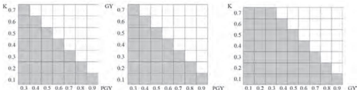
Figure 2: Ink combinations of printed patches; only combinations marked with gray are printed
