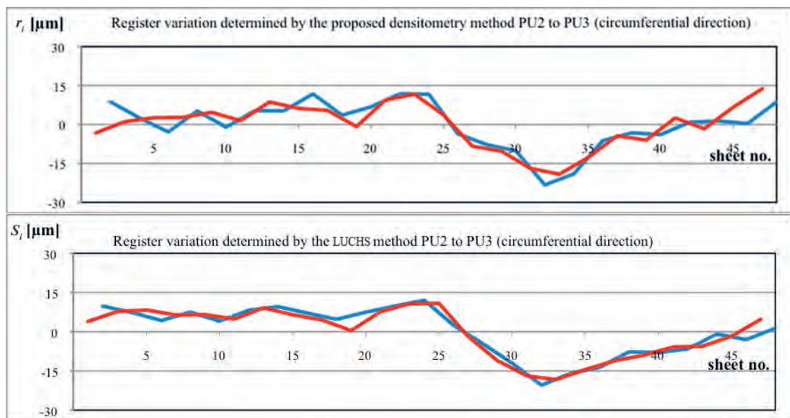
Figure 7: The comparison of the register variation graphics between the LUCHS ( $s_i$ ) and the proposed method ( $r_i$ ); the red curves demonstrate the odd and the blue ones the even results of the register position
