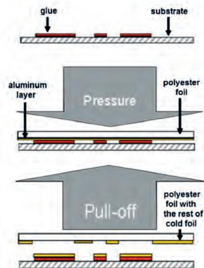
Figure 3: Working principle of cold foil transfer process (Heidelberg, 2012)
