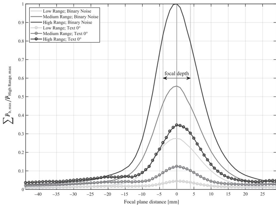
Figure 7: Power spectra of binary noise (solid lines) and text aligned at  $0^\circ$  (circled lines) test chart using Low, Medium and High Ranges of frequency bandwidths
